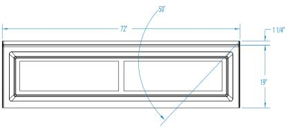
FEATURES Dimensional Tolerance ± 3/8". Dimensions needed for site preparation should be measured from the unit. Aquatic assumes no responsibility for preparatory work.
