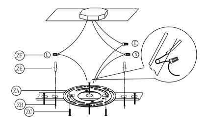
1. Drill two holes on the ceiling and put the plastic anchor screw(ZE) into the holes(If the wall is wood made, this step can be ignored);
