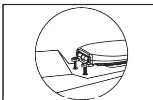
3. Check the fit of the toilet seat to the rim of the toilet bowl. Adjust the position of the seat if necessary.
