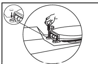
4. Tighten the bolts until the seat is securely attached. Install the plastic caps to cover the bolts.
