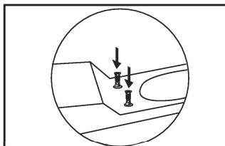
1. Insert the expansion anchors into the seat mounting holes on the top of the toilet bowl.
