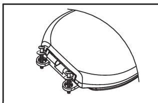
2. Insert the washers and bolts into the toilet seat installation holes.
