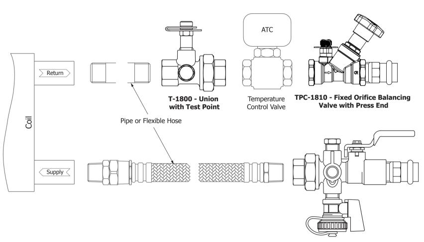
PCT-1830 - Combination Ball Valve with Drain, Test Point and Press End
