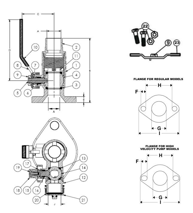
**Specifications:** Designed for residential, commercial or industrial use with water or a glycol mixture. This approved Webstone valve is actuated by a blowout proof stem and features an adjustable packing gland. Flange features a conical inlet to minimize turbulence. Solder joint temperature ratings are per ASME B16.18 Annex A for 95-5 solder. Other solder materials have lower pressure/temperature limits. Do not silver braze or over heat valves when soldering.
