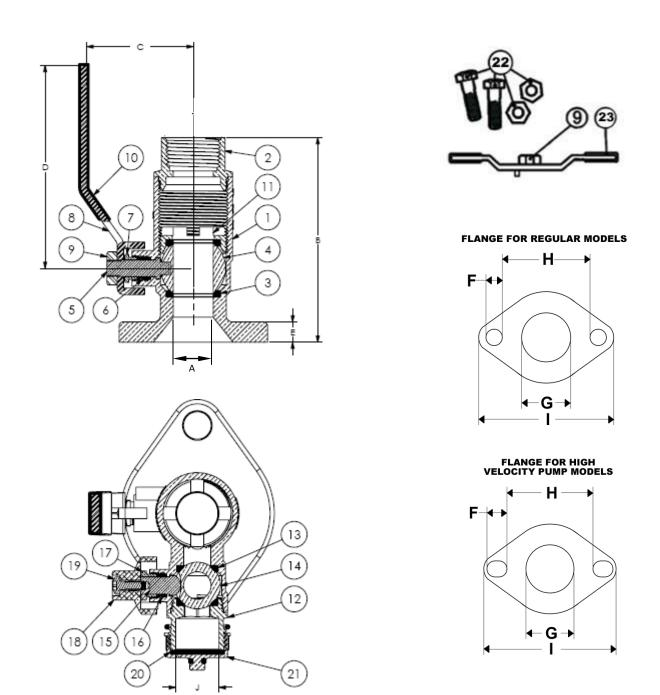
Specifications: Designed for residential, commercial or industrial use with water or a glycol mixture. This approved Webstone valve is actuated by a blowout proof stem and features an adjustable packing gland. Flange features a conical inlet to minimize turbulence. Threaded ends comply with ANSI B1.20.1.
